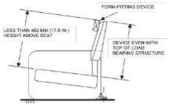
Test has been performed pulling the backrest backwards
